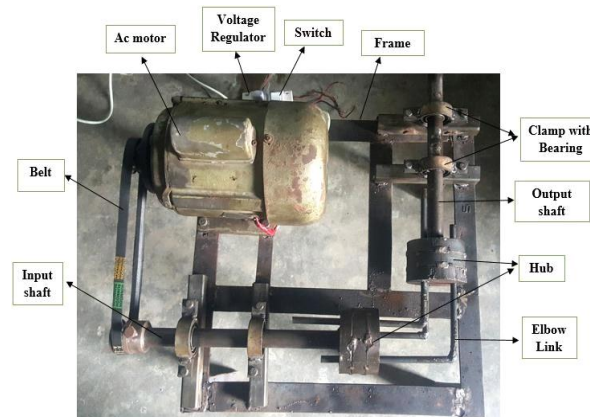
Fig. 4: Photographic view of Final setup of the project
